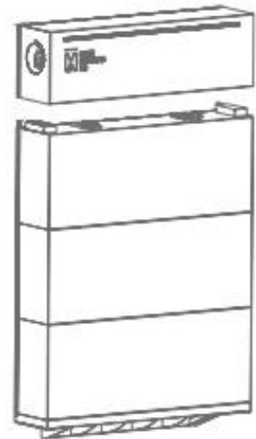
Assembled battery 196.5*800*315mm*N
